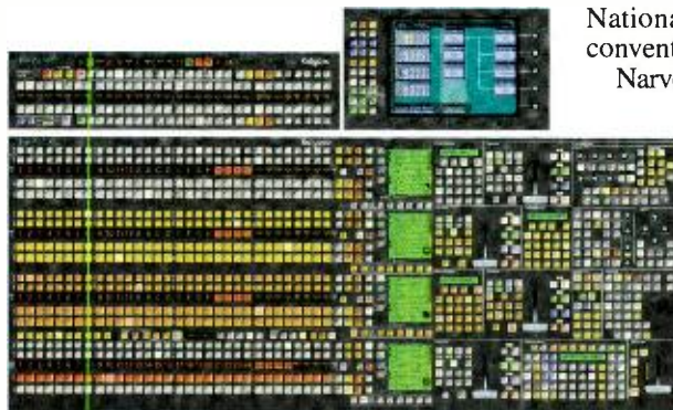
The Kalypso switcher includes six channels of integrated digital effects and can store video or stills.
