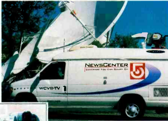
While wcvb-tv's van is equipped with a 40-foot mast, it is rarely raised for digital feeds. COFDM modulation allows wcvb-tv to send pictures from this 'DashCam' (inset) while the van is in motion at speeds of up to 60 mph.
