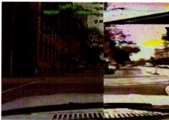
A side-by-side comparison of news feeds from NDS's COFDM system (l) and an analog FM system.
