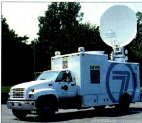
To uplink the game from Baltimore, Harris will use satellite truck it built for WJLA-TV Washington
