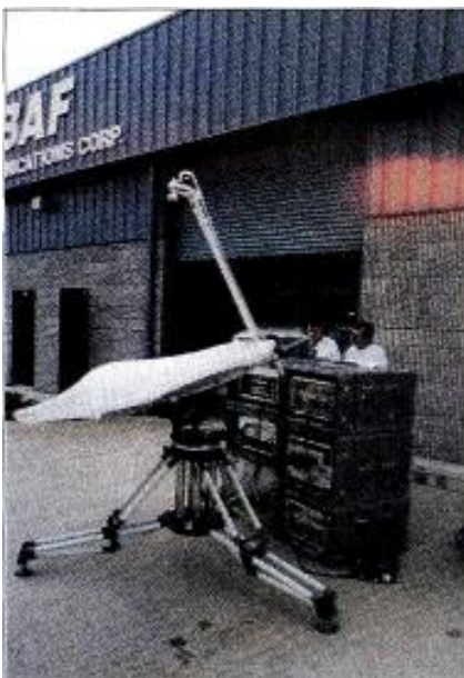
Above: Fox News's third SNG truck was put to work immediately. At left: The Fox Ku-band 'flyaway' package is a redundant RF uplink system.
