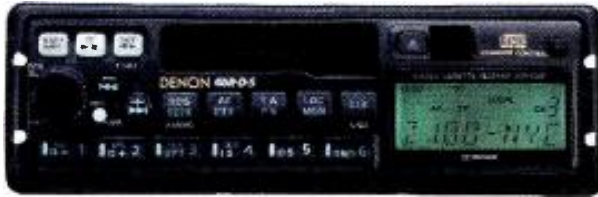
Denon's car audio system with RBDS; the display shows station slogan and city
