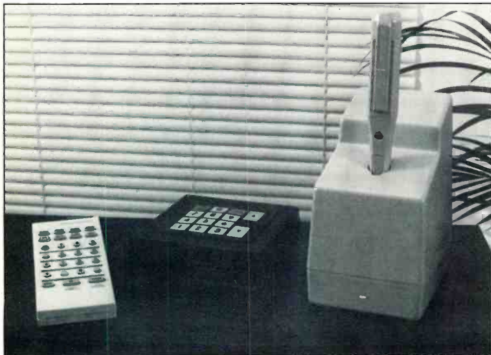
The three parts of Arbitron's local market single-source audience measurement are (from left): remote access keypad, data wand and meter which records information for overnight retrieval.
