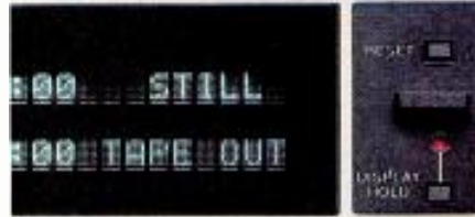
Display board for self-diagnostics and other data-processing functions.
