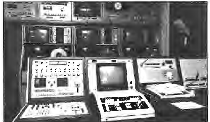
This is media center, which is essentially a post-production studio with seven one-inch VTR's, two two-inch VTR's and two film chains.
