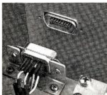
All leads to the deck go through this plug-in connector. There is nothing to disconnect to remove the deck.
