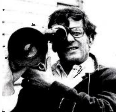
1. First step in KMOX-TV's electronic news-gathering system is portable Ikegami color camera, weighing less than 15 pounds.
