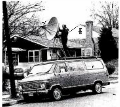
2. Stories can be transmitted to studio via microwave for immediate broadcast, or recorded on video tape within mobile unit.
