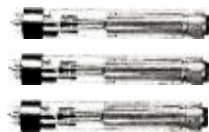
three lead oxide tubes in color channels
