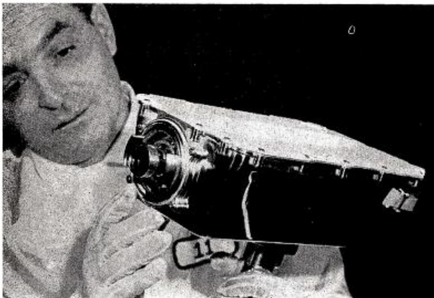
Westinghouse Electric Corp.'s Apollo moon camera, weighing only 7¼ pounds, will be carried by the first astronauts who explore the moon.
