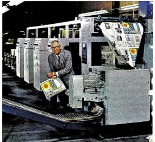
The Cottrell Model V-22 web offset newspaper press brings better printing and economical color to smaller newspapers. This one, owned by Industrial City Publishing Co., San Francisco, prints its four colorful weeklies with a combined circulation of 60,000.
