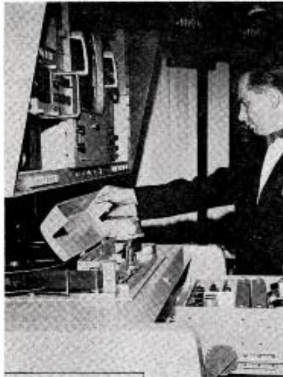
Visual Electronics' Sam Kichas lifts the panel of the Alienized tape TV recorder so heads are shown.
