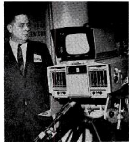
RCA's TK-33, black and white field camera, with demountable viewfinder, is explained by RCA demonstrator.
