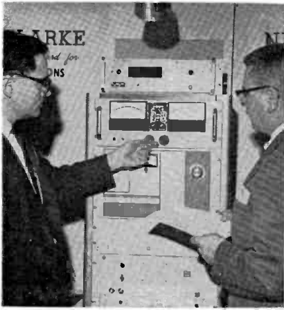
Vitro's John Birch changes control of phase meter which is reading out factors from transmitter over pair of telephone lines as Ogden Prestholdt, CBS Radio, New York, looks on.
