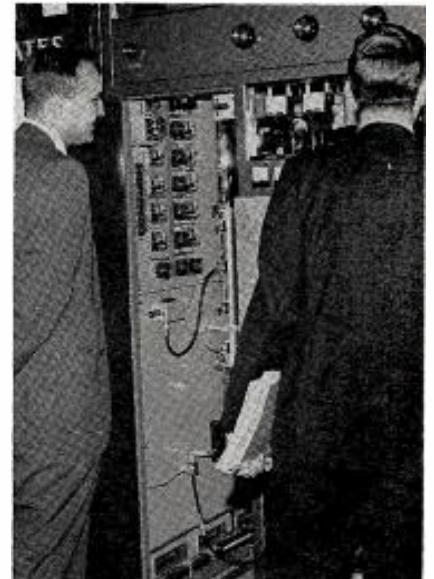
Couple of broadcasters look over innards of Townsend Associates 50 kw UHF television transmitter.
