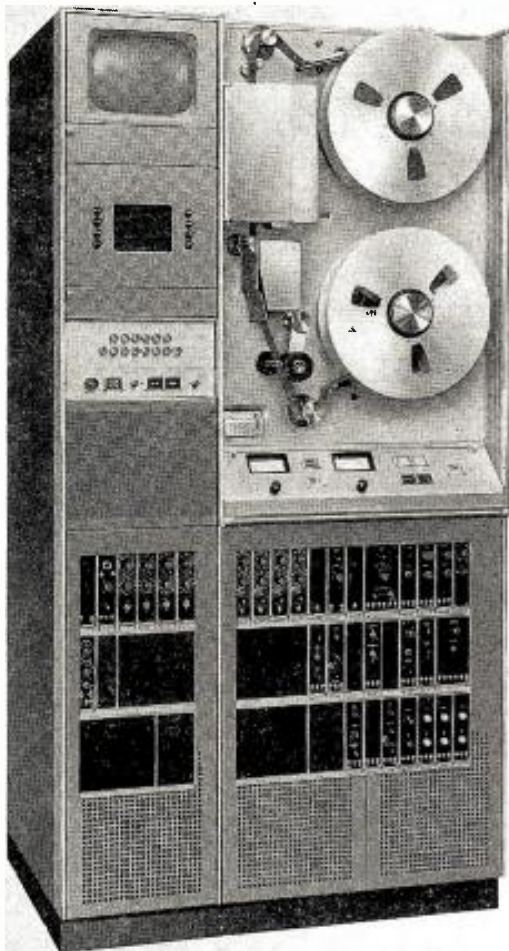
Modular layout of the TR-4 showing "record" group at left and "play" group at right.
