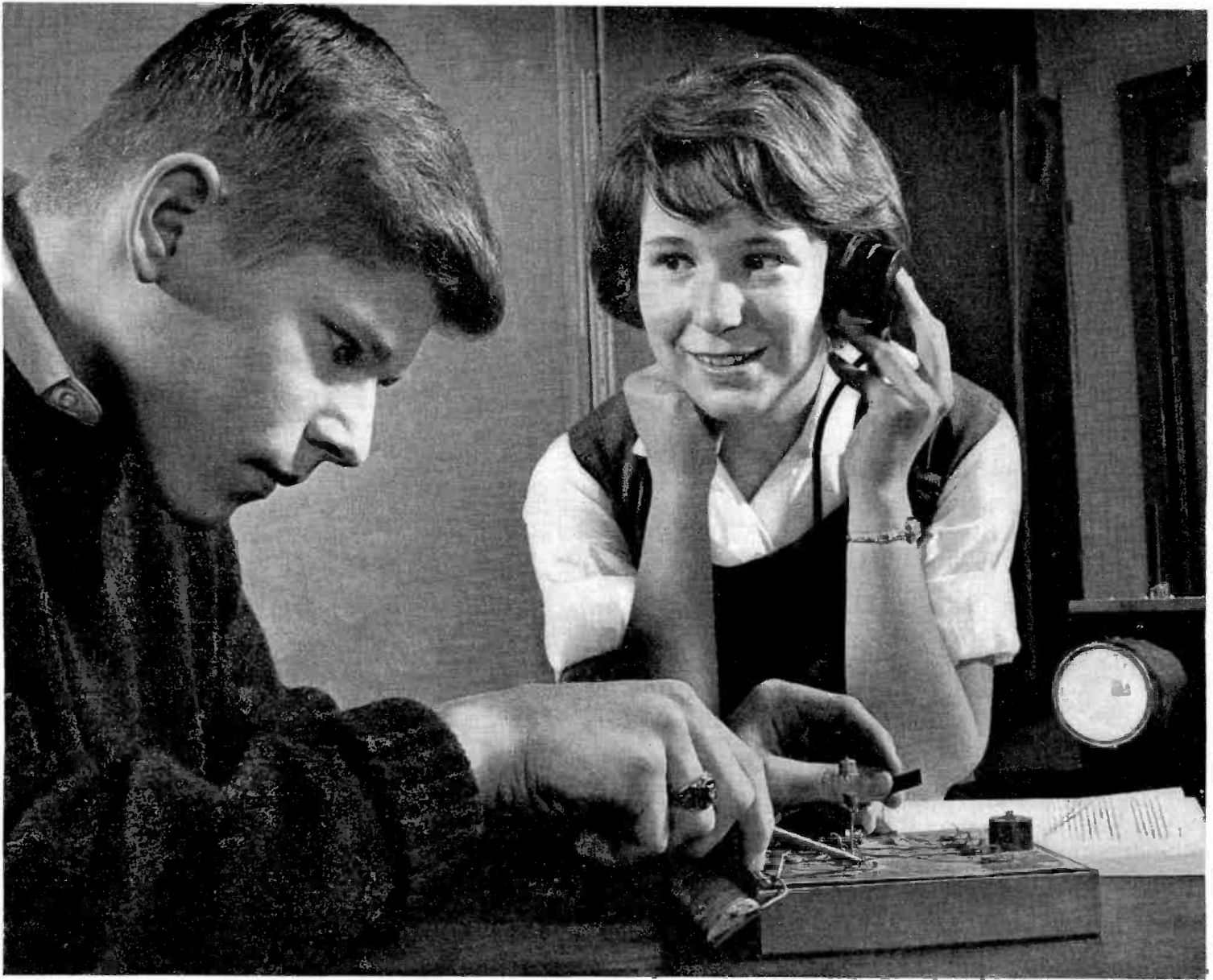
Two advanced physics students are producing a solar-powered, transistor audio-oscillator—the "From Sun to Sound" experiment—provided by the Bell System. The experiment requires students to calculate and design as well as construct some of the basic electronic components.
