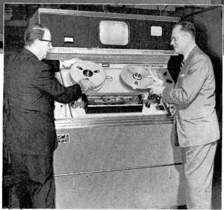
Frank Marx (R), Press., ABC Engineers, and Charles Colledge, V.P., RCA Broadcast and Communications Division, load up one of ABC's new total solid-state TR-22's.
