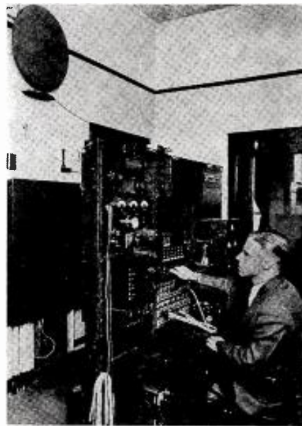
This was the console used in the WAPI Birmingham control room during the 1920's. Engineer Clayton Dow is riding the gain.
