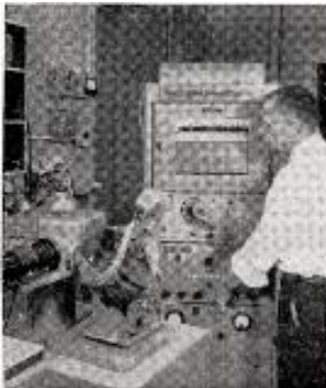
X-ray fluorescence spectrography, an advanced technique for the analysis of the compositions of alloys, provides quick answers to help speed laboratory projects.
