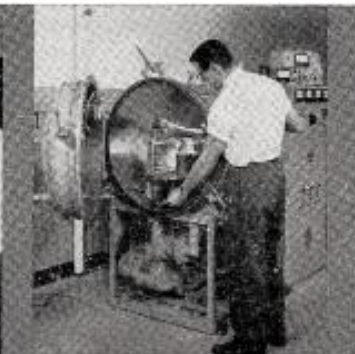
Vacuum melting techniques, which have made important commercial contributions in other fields, being studied to determine their effects on copper and copper alloys.
