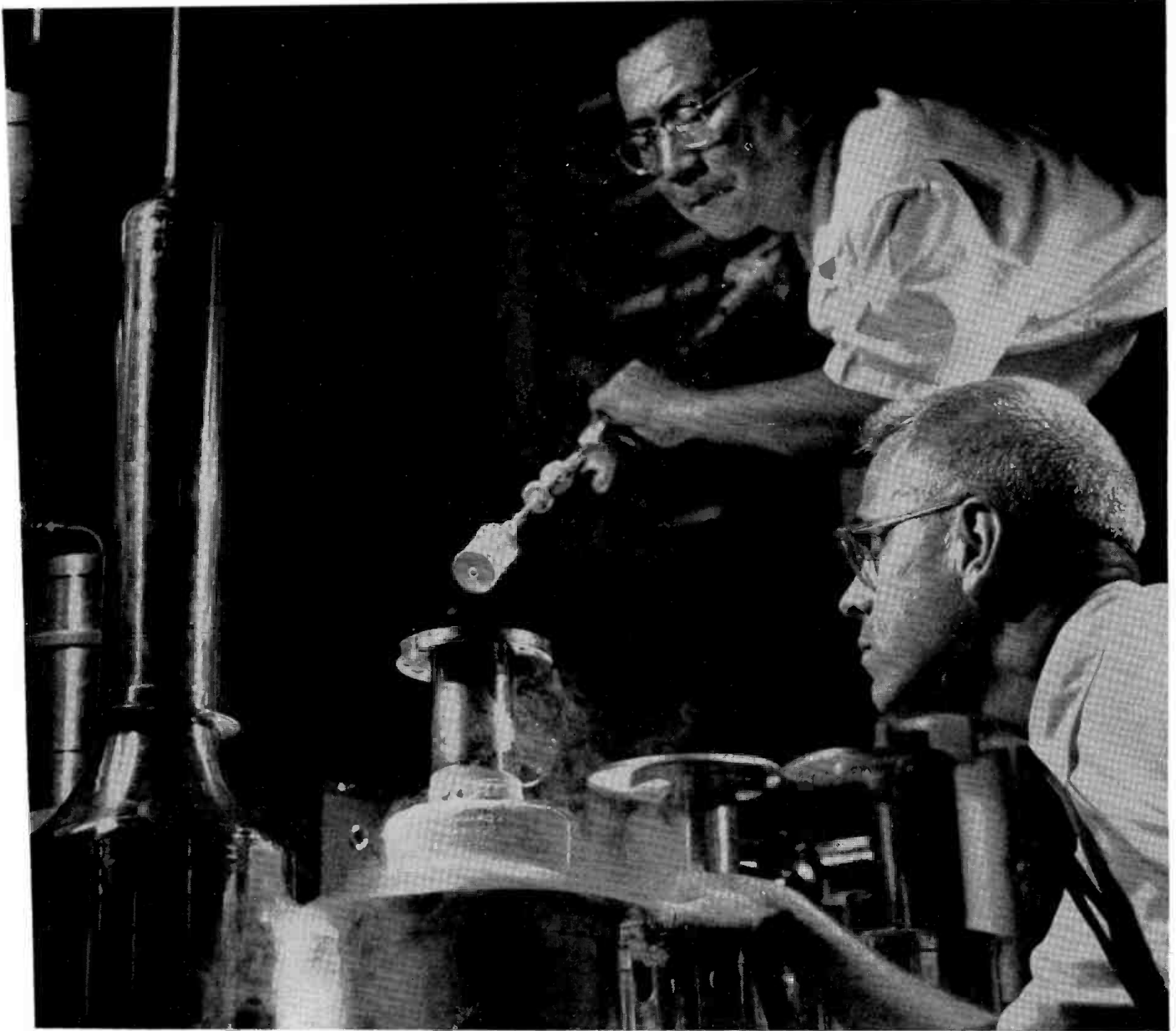
The Making of a Magnet. Bell scientists test new superconducting magnet. It's the small cylindrical object being removed from helium bath at 450° F below zero.
