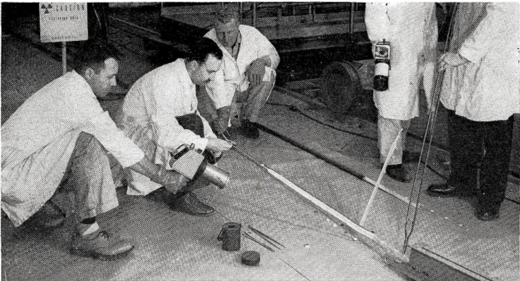
Clayton McDole, U.S. Steel scientist (second from left) supervises the removal of irradiated foil samples from General Electric Test Reactor. Information obtained provided a solid flux data foundation for the irradiation research of special reactor steels.
