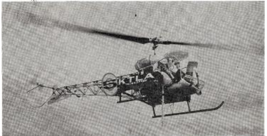
THIS is KTLA (TV) Los Angeles' new flying tv unit, the Telecopter [STATIONS, July 28]. The $42,000 Bell D-2 helicopter is equipped with audio and video transmitters, monitor, communications system, power supply and a GE Vidicon camera with Zoomar lens. Cost of developing and equipping KTLA's airborne news arm was about $40,000.
