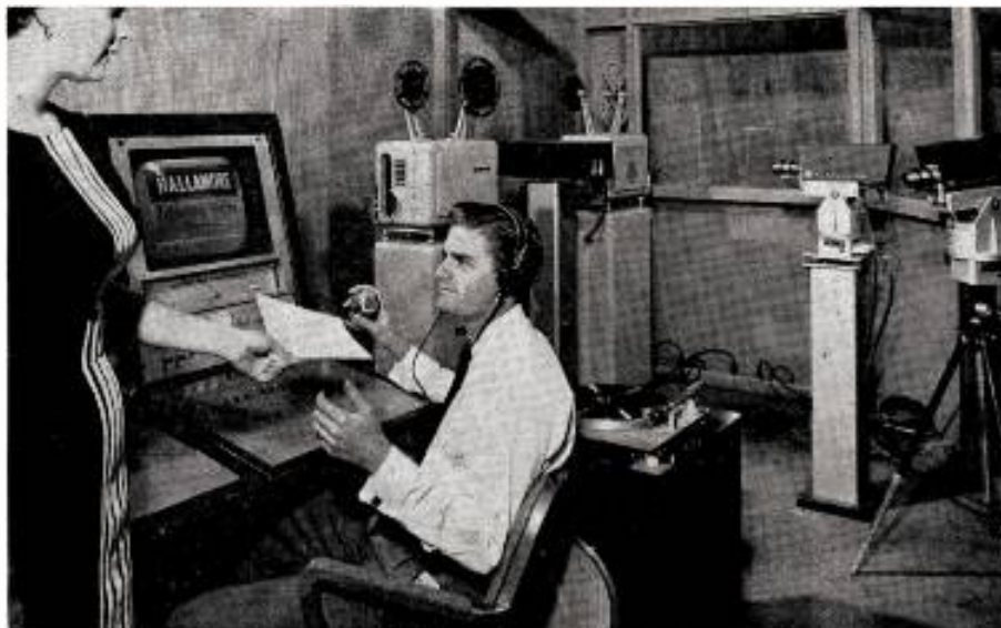
THE MAN and the machine are the television studio . . . or they now can be, with the components pictured of the new Hallamore tv origination unit. Seated at the master control console, the announcer can control and monitor all the elements of the unit, with the dials and switches of the control console taking over the former province of the engineer.
