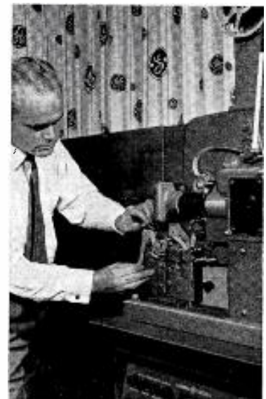
Film threading of the Eastman Continuous Motion 16 mm Projector is fast and easy. Light compensating mirrors, behind window, are out of the focal plane—eliminating dust problem—and rotate at 770 rpm.
