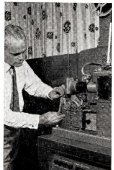
Film threading of the Eastman Continuous Motion 16 mm Projector is fast and easy. Light compensating mirrors, behind light window, are out of the focal plane—eliminating dust problem—and rotate at 770 rpm.
