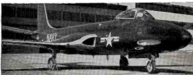
Built-In Hole. Behind the gun opening on this jet interceptor is a "blast tube," to protect the plane from high pressures and gases caused by the firing of the gun. Formerly, this tube was machined from solid steel bar stock, but has now been replaced with USS Stainless Seamless Tubes. These tubes are pierced from solid steel, and they afford the absolute uniformity of wall strength required.
