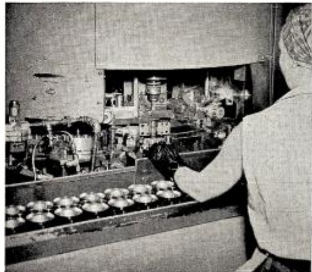
Boring the inside diameter of the hydraulic valve lifter body in preparation for a honing operation.
