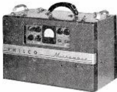
Transmitter Control and Power Supply
