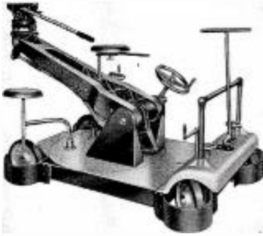
PANORAM DOLLY gives camera complete mobility; smooth panning, dolly shots, running shots, special effects. Two man crew.
