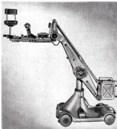
MODEL BT-1 CRANE has power drive, hydraulic lift. Provides lens height from 2' to 10'. Developed for Motion Picture Research Council.
