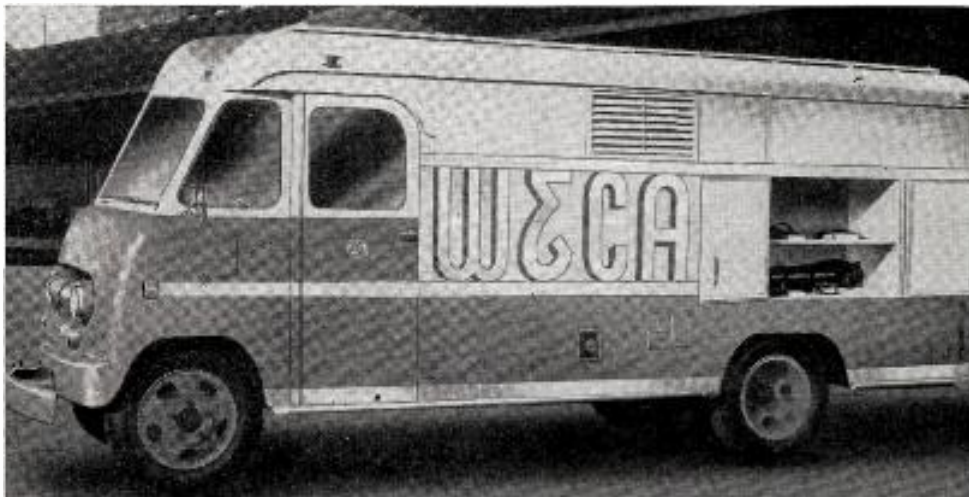
NEW type TJ-53A mobile TV unit developed by RCA Victor's Engineering Products Dept. and priced at $11,400, will carry all equipment needed to pick up, monitor and relay remote TV events to a video station, the firm announces. It contains an air-conditioned control room with facilities for driver, program director and three technicians, and storage space to carry three field TV camera chains plus operating equipment.
