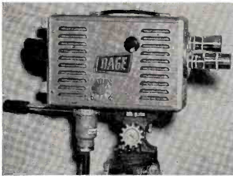
THIS is Dage Electronics Corp. new portable TV camera weighing less than 20 pounds.
