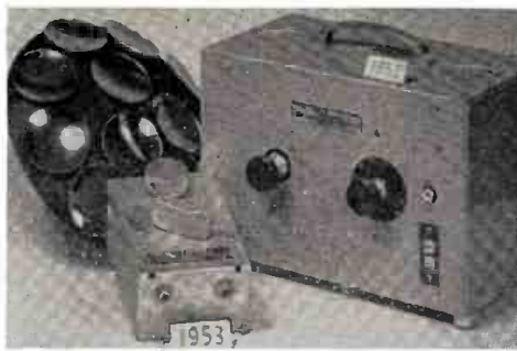
NEW synchronizer (below) of Musicolor Inc. greatly reduced in size from 1952 model (right) through use of transistors. At left is concave mirror rotor.
