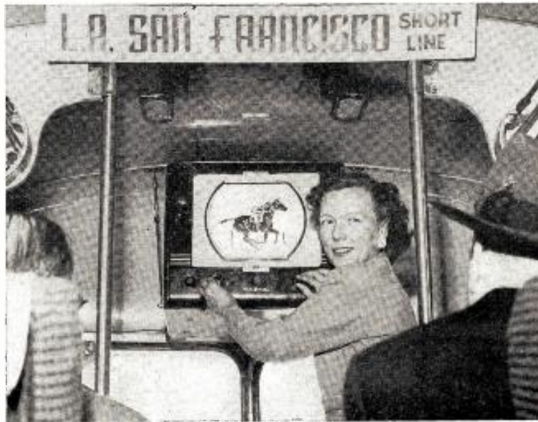
INSTALLATION of RCA Victor sets on Airline Bus Co.'s Los Angeles to San Francisco "Short Line" runs marks inauguration of transit TV in California. Gladys Hoffman, of San Francisco, adjusts set prior to the bus line's first TV trip. Line reported receiving programs up to 75 miles from point of origination on the initial run.
