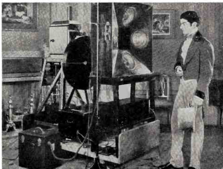
Mechanical scanning equipment, used at RCA-NBC experimental television station W2XBS in 1928, long before the RCA image orthicon camera.
