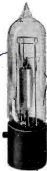
1918. This "peanut" tube, the Western Electric 215A, was developed for service in World War I. It was the first commercial tube whose filament was powered by a single dry cell. It made possible compact, light weight radio equipment.
