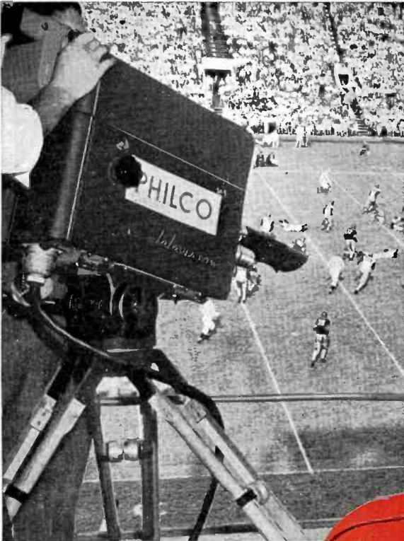
RCA image-orthicon cameras, standard equipment for the new truck, rival the human eye in sensitivity—eliminate fading of sports events. Shown above as used by Philco's WPTZ to pick up a Penn game at Franklin Field, Phila.
