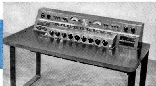
1946. The 25B console is an improved, enlarged version of the 25A, introduced in 1942. For either FM or AM use, the 25B provides two channels and controls two FM or AM programs simultaneously. This new equipment is compact, rugged and modern in appearance. Ease of control, instant accessibility, plug-in cable connections and a frequency response of \pm 1 db, 50 to 15,000 cycles are some outstanding features.
