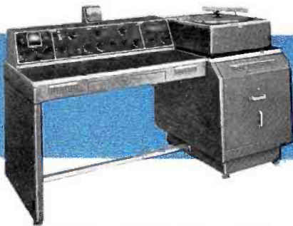
1939. This custom-built audio console for WOR was the first commercial type meeting all requirements for FM use. It provided circuits and equipment to meet specific operating conditions. The tailored metal desks mounted amplifiers, control and switching equipment and turntable units—all within easy reach of the operator.
