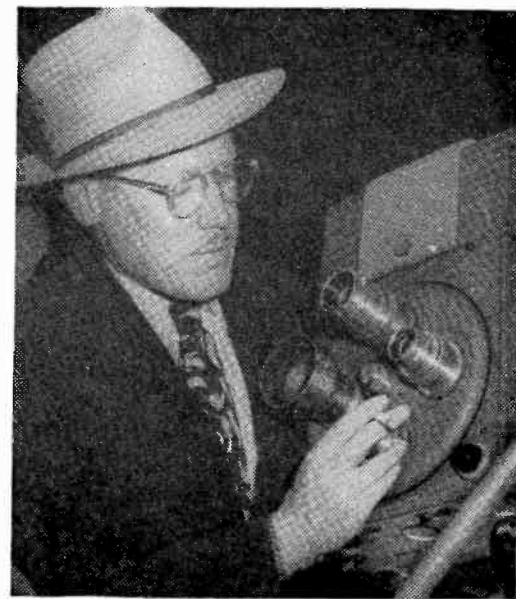
BURKE CROTTY, who directed Louis-Conn fight production at Yankee Stadium, examines one of the two new RCA Image Orthicon cameras equipped with turret-lens assembly.
