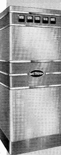
Complete 250 Watt FM Transmitter. This unit is also used as the exciter for higher powered transmitters.
