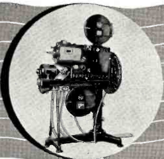
9. THE FILM SCANNER — The arrangement which allows standard motion picture films (24 frames) to be televised over a 30-frame, interlaced system was devised by RCA engineers.
