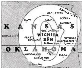
Clarence D. Gillies Computed Field Strength Distribution Based on Performance and Previous Survey Measurements—5000 Watts Day and Night—October 1941
