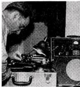
CLAMP-ON LIGHT, the idea of Clifton Todd, chief engineer of WNAX, Yankton, S. D., is hailed as a big help in adjusting the depth of cut on transcriptions. Here Engineer Todd is adjusting the cutting needle of WNAX's new recording unit.
