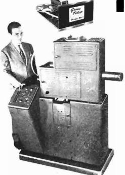
This most versatile telecasting optical projector enables dual projection with any desired optical dissolve under exact control.
