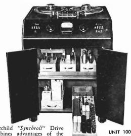
★ The Fairchild "Synchroll" Drive System combines advantages of the transfer of power through soft rubber idlers with those of direct gear control of the capstan. This unique development of Fairchild results in a no-slip synchronous tape drive.
