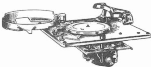
Figure 3. The components of the record changer are shown in this figure. The magnetic pickup's high tracking pressure and poor compliance must have resulted in a short record life.
