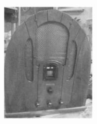
The delaminated front piece is re-glued, a new veneer piece installed and the remaining finish is removed by scraping and the missing moldings fabricated. The reassembling of the chassis meant emptying all the capacitor cans and the Bakelite blocks to fill them with new capacitors. The primaries of the damaged coils were rebuilt. The rebuilding of the tuning indicator required 10,800 turns of 0.071 mm wire and the adjustment of the movement was a challenge.
