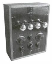
Federal Model 135 – This four tube receiver was made to fit into the cabinet of your replaced photograph. It was manufactured in 1924 by the Federal Telephone and Telegraph Co. of Buffalo, NY. Dave Crocker, Mashpee, MA.
