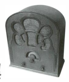
Freed-Eisemann Model NR-205 – This seldom 5 tube receiver of 1924 was produced was produced to replace your phonograph and fit into its cabinet. The controls were under the flip-top cover at the top. Dave Crocker, Mashpee, MA.
