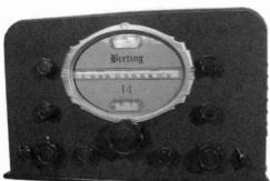
**Bretting model 14** – Manufactured in 1937. The frequency coverage is from 550 kc to 34 mc. It has 14 tubes and originally sold for \$100. Rudy Gertz, Omaha, NE
