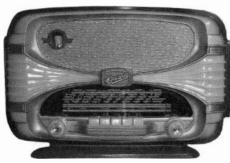
Oceanic radio – Model name Surcouf. Made in France in 1956 with a compliment of six tubes. Covers the AM and two shortwave bands. Donny Foster, Los Angeles, CA
