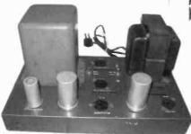
Eico HF-50 Audio Amplifier – The power output from this mono block audio amplifier was 60 watts. Output tubes are 2 x EL34. Made in 1959. The HF-50 used a Chicago output transformer and the HF-60 used a Accrosound output transformer with an output of 60 watts. Karl Breen, Fargo, ND
