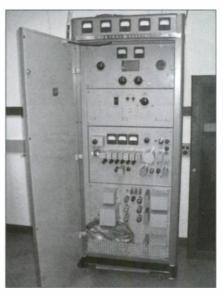
A General Electric type BT-1-B FM transmitter, circa 1940s. Output 250 watts, 88 MHz-108 MHz. It's still in operation.
