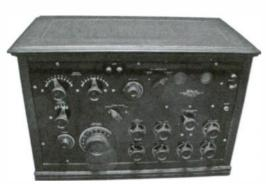
Federal model 61 radio – The model 61 was manufactured in 1924 by the Federal Radio & Telephone Company. It is a rare battery set with 6 tubes. The front panel is made of Bakelite and the top panel lifts. Morris Wonderling, Honolulu, HI
