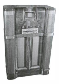
Airline model 62-403 console radio – This console was manufactured by Montgomery Ward in 1939. Features the "Movie Dial" and pushbottons. There are 13 tubes and covers the BC and SW bands. Bob Corwin, Gulfport, MS
