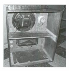
The rear of the custom-built tombstone cabinet showing the 10-inch speaker and the piece of Plexiglas I glued in place from the inside to protect the original Fisher dial scale glass on the chassis.
