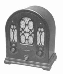
Atwater Kent model 165 – This wooden cathedral radio was sold by Atwater Kent in 1933. It uses a five-tube chassis and receives the broadcast band only. The grille decoration is very delicate. Dave Crocker, Mashpee, MA
