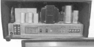
Fisher model 90-T - This is an AM/FM monotuner pre-amplifier manufactured approximately 1958. It features a tuning eye and inputs for phono, tape, aux 1, and aux 2. Arthur Morris, Englishtewn - NJ.
