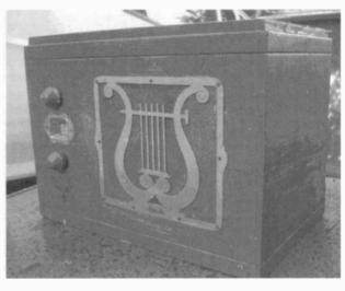
reception and sound quality is very good, probably the best of Smart Set series of radios, mainly because of the two IF stages and separated audio and AVC detection circuits. A 10-inch-long external antenna works very well, and I was able to pick up more than 15 stations on the AM band and every signal was clean, crisp and very clear. There was no hum, static or buzzing.
