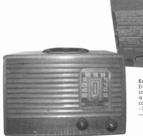
Emerson Model 425 - This nice wood-cased Emerson was manufactured in 1942 and comes with the original back cover. There is a plastic handle on top and the receiver covers the AM broadcast band. (Walter Green - Sharpsberg, PA)
