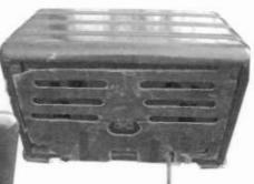
RCA 56X3 – Circa 1946, tube line up: 12SG7, 12SK7, 12SQ7, 35L6GT and 35Z5GT. Five-inch speaker has a nice tone. It is a very sensitive set, even though a simple one with just the broadcast band. Has high/low tone control. (Paul Buresh, Needham, MA)
