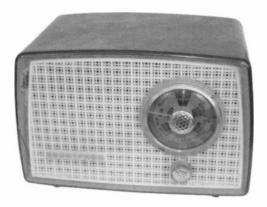
HORNYPHON "HORNYETTA" MODEL W147U - This 1957 Austrian radio was very popular because of its plastic cabinet and the fact that it worked with AC/DC and received MW. (Erwin Macho - Vienna, Austria)
