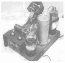
Figure 3. The simple construction of the Model 2-C-1'.s two-tube chassis with speaker removed.
