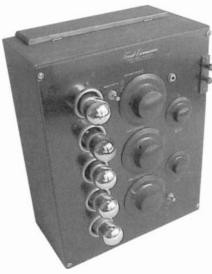
FREED-EISEMANN NR-102 – This 5-tube Neutrodyne was manufactured by the Freed-Eisemann Radio Corp. of Brooklyn, New York. It is a rarely seen 1925 radio, as it is one of only 70 produced. All five tubes stick out of the front panel in a vertical configuration. There is a wooden cover on the top that lifts and covers the binding posts which are factory-labeled on a card. (Dave Crocker – Mashpee, MA)
