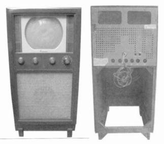
EMERSON MODEL 638 TELEVISION – Manufactured by the Emerson Radio & Phonograph Corporation in 1949. This television used a 10 inch CRT and a total of 22 tubes. The chassis was used in both table top and floor versions. (Mark Arkin, Los Angeles, CA)
