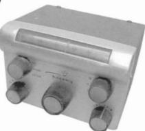
**REGENCY MODEL ATC-1** - This amateur band converter was manufactured by the Regency division of I.D.E.A., Inc. of Indianapolis, IN. It operates on a transistorized circuit for reception of the 80, 40, and 20 meter bands, and can be used with any broadcast receiver, either automobile, portable or home receiver. (Robert Enemark, Duxbury, MA).
